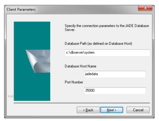
**Note** The **Database Host Name** and **Port Number** values provide the TCP/IP information for the client to connect to the server. The **path** parameter is specified from the perspective of the database server, and not as a mapped network drive from the perspective of the standard client.
