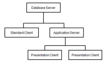
A database server must run a 64-bit Windows operating system. An application server, standard client, or presentation client can run 32-bit or 64-bit Windows.
