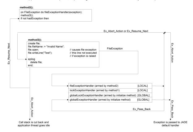
Referring to the above image, you will observe that when the **fileExceptionHandler** (armed by **method2**) returns **Ex\_Abort\_Action**, the epilog is executed. When this has been performed, the call stack is cut right back (performing each method's epilog as the stack is cut back), and the application essentially goes idle.
