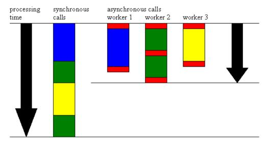
The red section of the bar represents the time utilized by the framework to manage the asynchronous method calls
