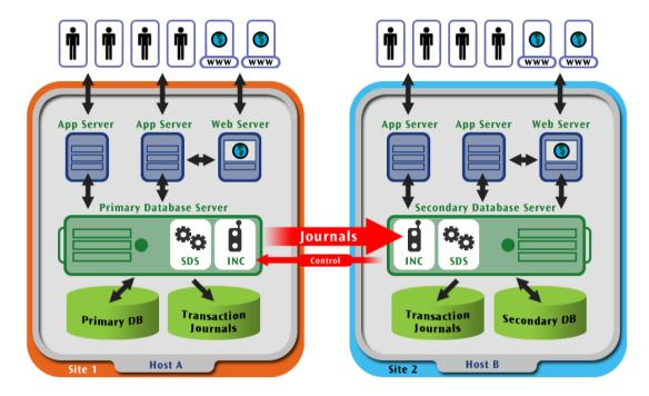
The above image of active hot-standby configuration illustrates the deployment of a single secondary database server operating in an active 'hot standby' mode. The secondary server is installed at a different location to the primary. In this example, the secondary database provides a remote 'hot standby' database while at the same time supporting read-only database access.
