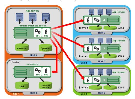
The above image of hybrid multiple secondary configuration illustrates an SDE comprised of multiple secondary database servers. This more-complex scenario combines the passive standby functionality from example 1 with the active remote standby functionality from example 2 and introduces the use of multiple read-only secondary servers for application load-balancing.
