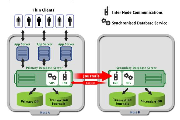
The above image of passive hot-standby configuration illustrates a single secondary database server operating in a passive 'hot standby' mode. SDS is an integral component of a database server node; the above image illustrates some of the key components of this service. The Inter Node Communications module (or INC) transports the messages used by SDS to communicate between database servers.
