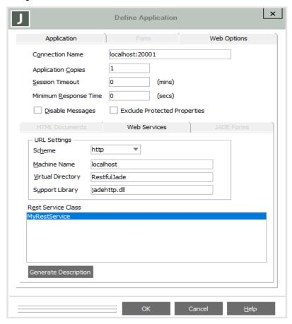
This application is the entry point into the JADE database and calls the **processRequest** method of the specified **JadeRestService** class subclass whenever a request is received on the port specified in the **Connection Name** text box.
