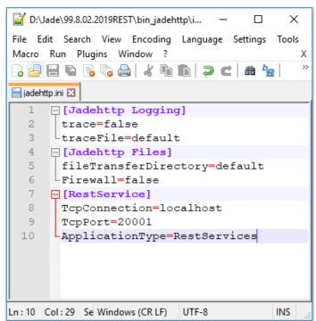
**Note** The **TcpPort** parameter value can be any unused port, but it must match the port number specified in the **Connection Name** text box on the **Web Options** sheet of the Define Application dialog for the JADE Rest Services application.
